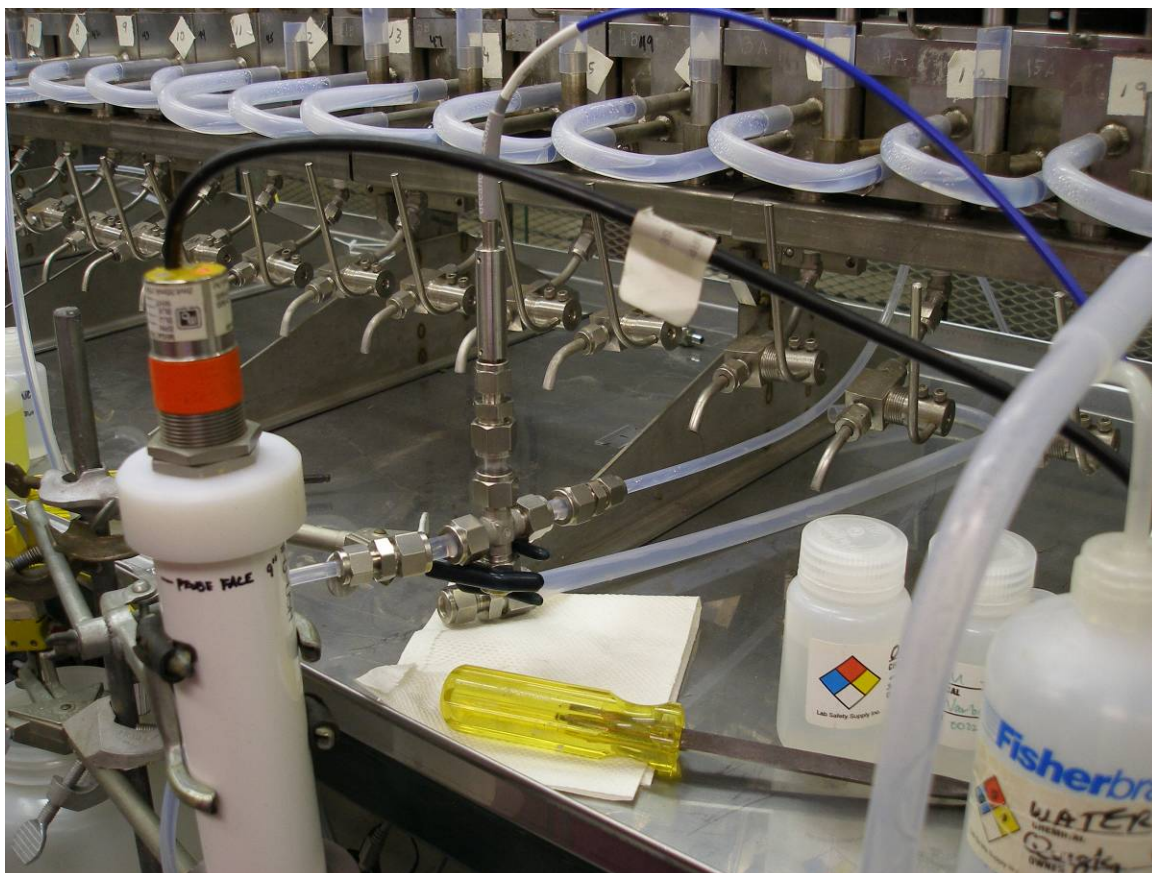
Figure 23: Fiber optic dip probe mounted in aqueous product outlet
