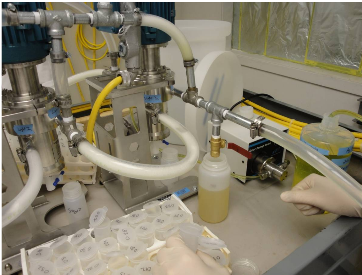
Figure 37: Foaming in organic interstage tubing
